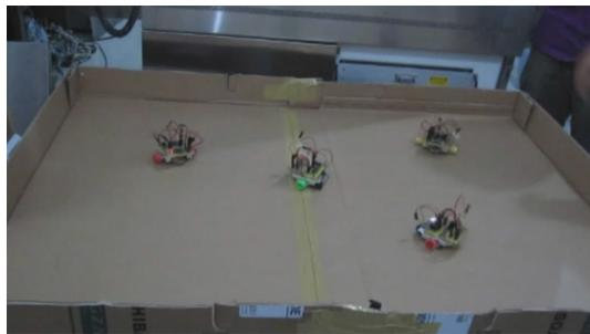
**Fig. 6.** Simulation Trial Demonstrating the Random Walk Routine
