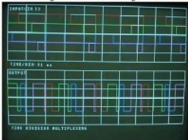
Fig. 23 Waveform output of time division multiplexing
