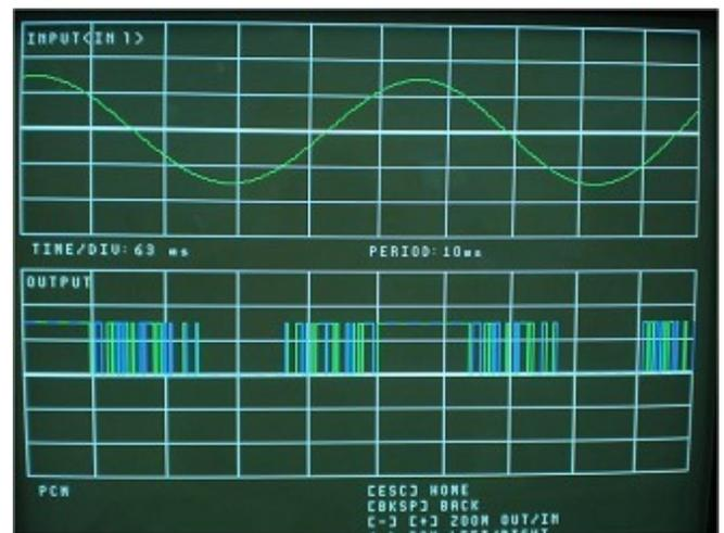
Fig. 18 Waveform output of pulse code modulation
