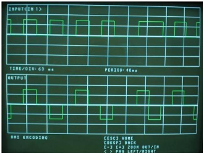
Fig. 22 Waveform output of alternate mark inversion
