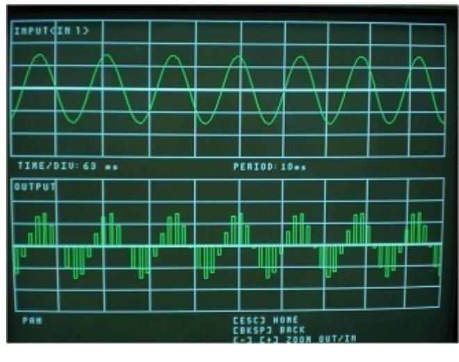
Fig. 17 Waveform output of pulse amplitude modulation
