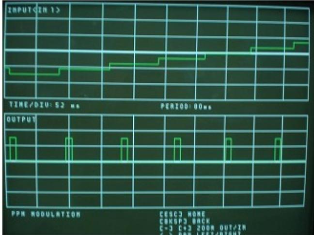
Fig. 19 Waveform output of pulse position modulation
