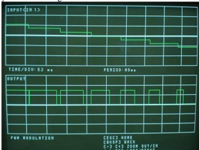
Fig. 20 Waveform output of pulse width modulation
