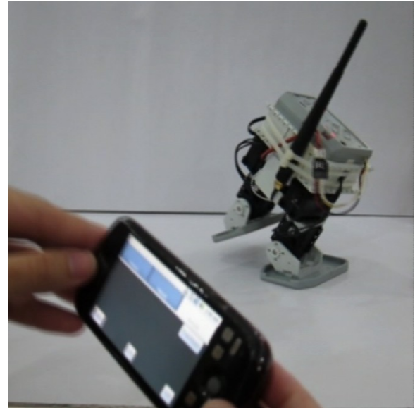
Fig. 7. The Google Android powered HTC Magic manipulating the robot using the accelerometer and geomagnetic sensor.
