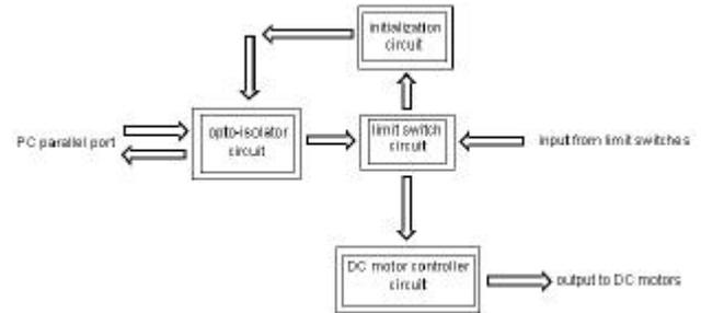
Figure 7. Block Diagram of the Controller Circuit Connections.
