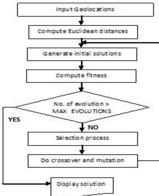
Fig. 2 Block Diagram of the Genetic Algorithm Implementation
